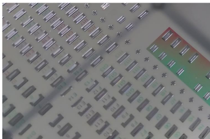
ICON Photonics structures integrated on a wafer
